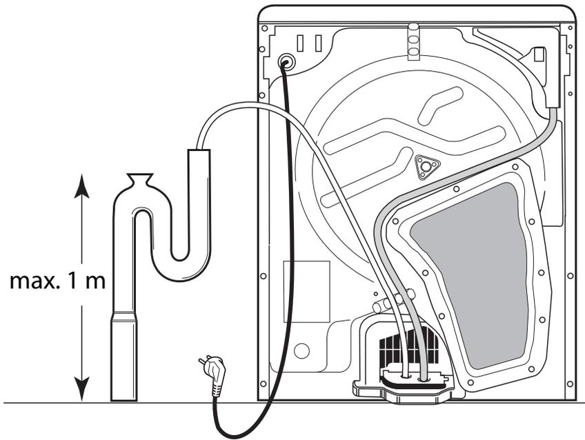
**NOTE:** To avoid siphoning, the end of the hose must not be immersed in the drain water. Avoid bending and twisting the hose.
