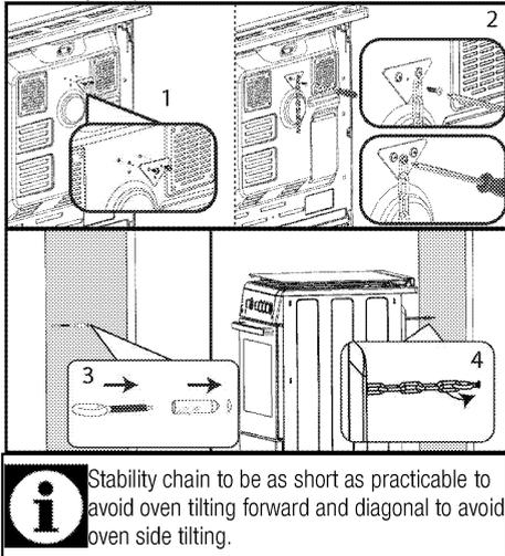
Cooker stability chain for cookers is not designed with bracket engagement slot.
