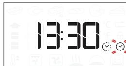
If necessary, turn the knob to set the time you want cooking to end, then press to confirm and start the function.
