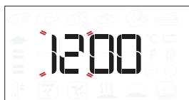
The two digits for the hour will start flashing: Turn the knob to set the hour and press to confirm.
