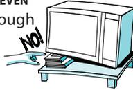
**P**osition the oven at a distance from other heating sources. For sufficient ventilation there must be a space of at least 30 cm above the oven. Ensure that the space underneath, above and around the oven is empty to allow for proper airflow. The microwave oven shall not be placed in a cabinet. This oven is not intended to be placed or used on a working surface lower than 850 mm above the floor.
