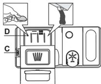
To open the detergent dispenser use the opening device C. Introduce the detergent into the dry dispenser D only. Place the amount of detergent for pre-washing directly inside the tub.
