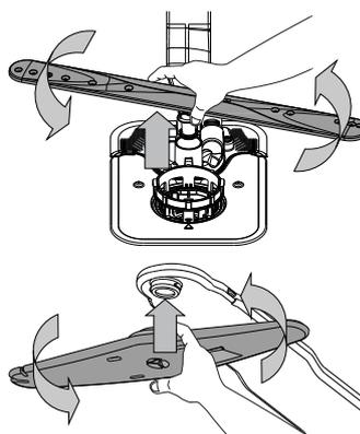
The lower spray arm may be removed by pulling it upwards and rotating it anti-clockwise. Mounting back the spray arm is by pulling it down and rotating it clockwise.
