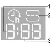
1. **Delay Time on the floor** - indicator of the time left to the start of the cycle, when the Delay option is set
