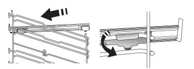
Please note: The sliding runners can be fitted on any level.
