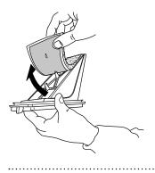
4. Clean the filter foam and the filter by hand or under running water. Do not wash the filter foam in the washing machine.
