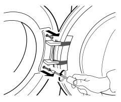
4. Remove the door and carefully lay it upside down on a blanket or similar.
