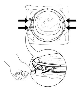
**10.** Remove the 4 inner screws on each side of the door.
