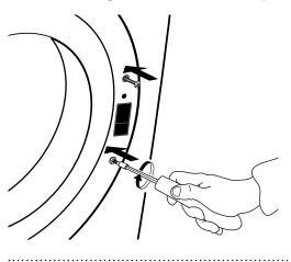
**20.** Fix the door on the left side of the door opening by turning in the two screws.
