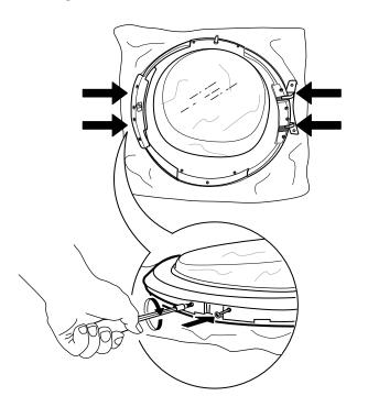
**14.** Fix the 4 inner screws on each side again.
