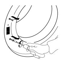
**2.** Press the small knob above the door lock with a small screwdriver. At the same time move upwards the door lock and pull it towards you with your finger.
