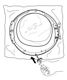
18. Insert the door lock on the right side of the door opening. Press it completely inside the hole and move it a bit downwards, until the small knob of the door lock latches.
