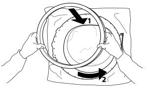
17. Turn the door again and lay it upside down. Fix the bottom screw again.
