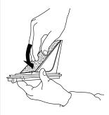
**7.** Clean the filter chamber of the dryer with a damp cloth or carefully with a vacuum cleaner.
