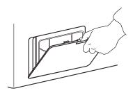
**2.** Hold the handle and pull out the bottom filter.
