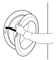
If you interrupt a running programme by opening the door, the programme will be reset if the dryer door is not closed again within one minute.
