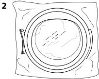
**7.** Carefully turn the door frame in clockwise direction, and remove it.
