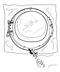
**6.** Turn the door and lay it down on the door glass.
