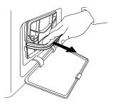
**3.** Remove the foam from the bottom filter, to clean it.
