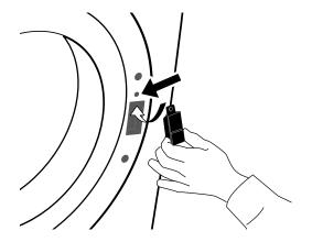
19. Fix the two screws over and under the door lock, on the right side of the door opening.
