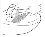
**5.** Carefully wring out the filter foam. Do not insert it in the bottom filter dripping wet.
