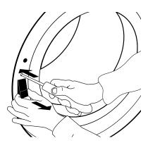
**3.** Remove the two screws on the door hinge.
