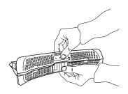
**3.** Carefully remove the complete lint from the screen by hand.
