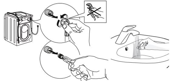
4. Insert the mesh filter again. Connect the inlet hose to water tap and washing machine again. Do not use a tool to connect the inlet hose. Open the water tap and check that all connections are tight.
