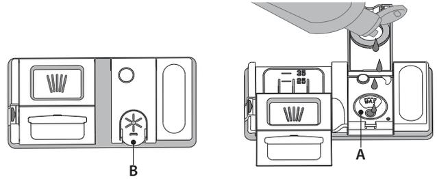
1. Open the dispenser **B** by pressing and pulling up the tab on the lid.
