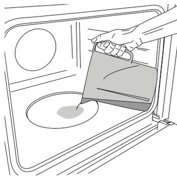
Only when the oven is cold, fill the embossing of the cavity with the quantity of drinking water suggested in the relative cooking table. Place the food in the oven.
