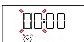
Use + or - to set the hour and press ○ to confirm. The two digits for the minutes will start flashing. Use + or - to set the minutes and press ○ to confirm.
