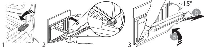
Put the door to one side, resting it on a soft surface. Refit the door by moving it towards the oven, aligning the hooks of the hinges with their seating and securing the upper part onto its seating. Lower the door and then open it fully. Lower the catches into their original position: make sure that you lower them down completely. Try closing the door and check to make sure that it lines up with the control panel. If it does not, repeat the steps above.
