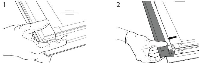
Lift and firmly hold the inner glass with both hands, remove it and place it on a soft surface before cleaning it.
