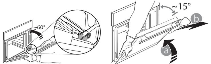
**3.** Refit the door by moving it towards the oven, aligning the hooks of the hinges with their seating and securing the upper part onto its seating.
