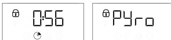
Once the cycle has been completed, the door remains locked until the temperature inside the oven has returned to a safe level. Air the room during and after running the Pyro cycle.
