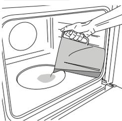
To start the Steam function, pour 200 ml of drinking water in the oven bottom. Select the function turning clockwise the selection knob on the relevant icon, and the thermostat knob in any position between 160 and 180°C (as suggested by the icon). The function will start and the display
