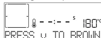
When the display shows the relevant message, if required press  to start a five-minute browning cycle. You can stop the function at any time by pressing  to switch the oven off.
