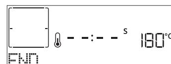
Press  to continue cooking in manual mode (untimed) or press + to extend the cooking time by setting a new duration. In both cases, the cooking parameters will be retained.
