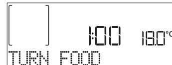
An audible signal will sound and the display shows the action to be done. Open the door, do the action prompted by the display and close the door, then press  to continue cooking.
