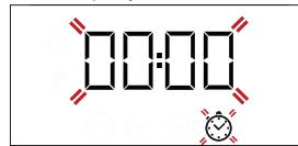
Use or to set the time you require and press to confirm. An audible signal will sound once the timer has finished counting down the selected time.
