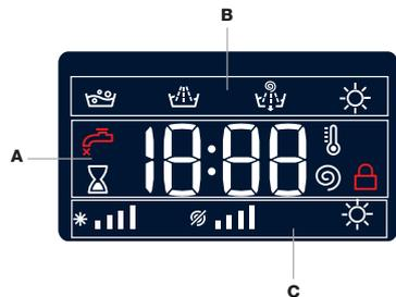
Section **A** displays the duration of the various available wash cycles and, once the cycle starts, the time remaining to the latter's end (the display will show the maximum duration of the selected cycle which may decrease
