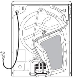
If possible you can drain the water directly into the domestic plumbing system. This will avoid having to empty the water container at the end of each drying cycle since the condensation water can be directly drained away (see chapter DRAINAGE SYSTEM).
