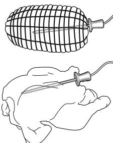
It is very important to position the probe accurately in order to obtain perfect cooking results. Insert the probe fully into the fleshiest part of the meat, avoiding bones and fatty parts. For poultry, the probe should be inserted sideways, in the middle of the breast, taking care to ensure the tip does not end up in a hollow part. In the case of meat with very irregular thickness,
