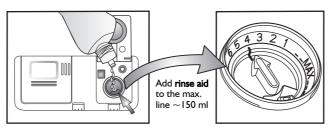
The rinse aid dosage can be adjusted to the detergent used. The lower the setting, the less rinse aid is dispensed (factory setting: position 4). Press the button to open the cover B. Using a coin or similar object, turn the arrow to the desired setting. After adjusting the rinse aid setting, shut the cover again.
