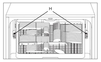
**How to remove cutlery rack** (if available) - It could be useful to remove cutlery rack to load stem glasses in upper rack.
