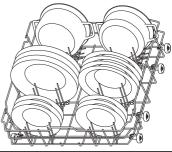
Arrange crockery so that water does not collect in cavities, ensuring that the spray arms turn freely. Only use dishwasher-proof crockery and dishes. Do not use the dishwasher for washing wooden items, aluminium, tin, silver cutlery or decorated crockery (unglazed). In the baskets, dishes (e.g. plates, bowls, pots) must be placed in a correct way to let water flow down!
