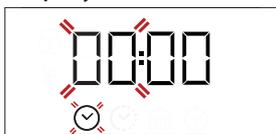
Use + or - to set the hour and press to confirm. The two digits for the minutes will start flashing.
