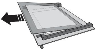
**3.** Refit the intermediate pane (marked with "R") before refitting the inside pane: To position the panes of glass correctly, make sure that the "R" mark can be seen in the left-hand corner. First insert the long side of the glass marked "R" into the support seats, then lower it into position. Repeat this procedure for both panes of glass.
