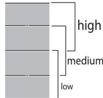
The flexible zone is divided into three cooking zones (see the figure) activated at a pre-set power (high, medium or low) depending on the position of the pot/pan: move the pot/pan over the surface to continue cooking at different temperatures without having to use the controls.
