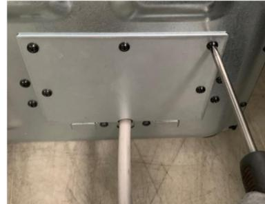
Assemble cover and tighten screws.
