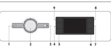
Start delay activated 🖓 Key lock activated ----Washing phase 🖄 🌾 🖗 Indicates washing phase of the cycle Failure: Call Service (9) Refer to Troubleshooting section Failure: Water filter clogged 🌐 Water cannot be drained; water filter might be blocked Failure: No water 😤 No or not sufficient inlet water.
