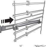
Remove the shelf guides from the oven and remove the protective plastic from the sliding runners.
