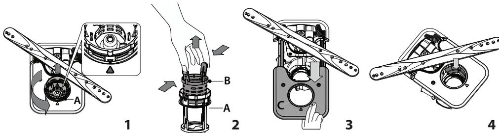
**The dishwasher must not be used without filters or if the filter is loose. It is important when reinstalling the filter that the two triangles shown on the zoom meet (Fig 1).** In case you find foreign objects (such as broken glass, porcelain, bones, fruit seeds etc.) **please remove them carefully.** Inspect the trap and remove any food residues. **NEVER REMOVE** the wash-cycle pump protection (shown by an arrow) (Fig 4).
