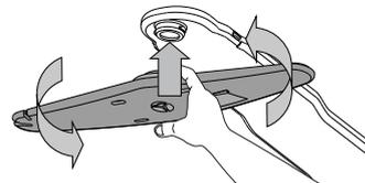
The ceiling spray arm may be removed by pressing it up and then rotating it anti-clockwise. Mounting back the spray arm is by pulling it upwards and rotating it clockwise.
