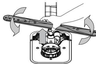
The lower spray arm may be removed by pulling it upwards and rotating it anti-clockwise. Mounting back the spray arm is by pulling it down and rotating it clockwise.
