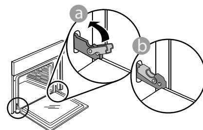
Apply gentle pressure to check that the catches are in the correct position.
