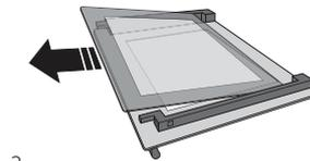
To correctly reposition the inner glass, make sure that the "R" is visible in the left-hand corner and the clear surface (not printed) is facing up. First insert the long side of the glass indicated by "R" into the support seats, then lower it into position (4). Refit the upper edge (5): a click will indicate correct positioning. Make sure the seal is secure before refitting the door.
