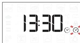
If necessary, turn the knob to set the time you want cooking to end, then press
