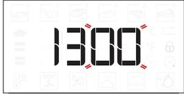
The two digits for the minutes will start flashing. Turn the knob to set the minutes and press **OK** to confirm.
