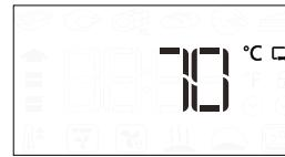
Press to start settings. Turn the knob to set the meat probe target temperature. Press to confirm. Turn the knob to set oven cavity temperature.
