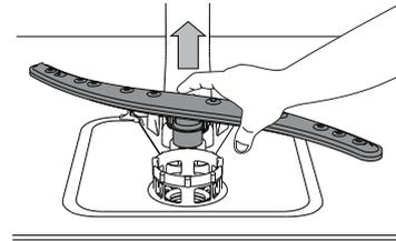
The lower spray arm may be removed by pulling it upwards.
