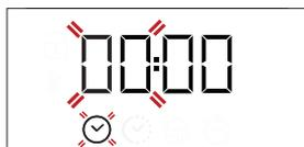
Use + or - to set the hour and press
