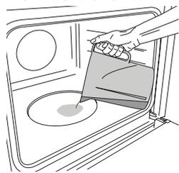
To start the Turn&Go Steam function, pour 200 ml of drinking water in the oven bottom. Select the function turning clockwise the selection knob on the relevant icon, and the thermostat knob in any position between 160 and 180°C (as suggested by the icon).
