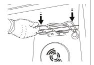
**3.** To reposition the heating element, lift it up, pulling it slightly towards you, making sure it comes to rest on the lateral supports.
