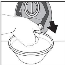
5. Turn the stopper of the "emergency drain hose" at the end of the hose and let the water flow into the container.
