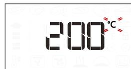
When the °C/°F icon flashes on the display, turn the knob to change the value, then press to confirm and continue to alter the settings that follow (if possible).
