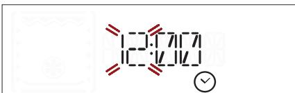
Turn the *adjustment knob* to set the correct hour and press
