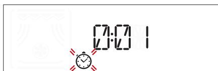
Press **OK select** to activate the timer: An audible signal will sound and the display will indicate once the timer has finished counting down the selected time.
