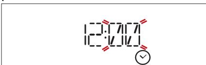
Turn the *adjustment knob* to set the minutes and press
