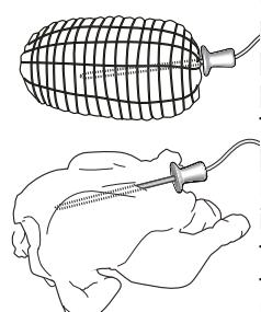
It is very important to position the probe accurately in order to obtain perfect cooking results. Insert the probe fully into the fleshiest part of the meat, avoiding bones and fatty parts.
