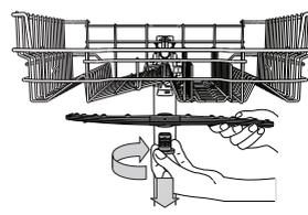
To remove the upper spray arm, turn the plastic locking ring in a clockwise direction.
