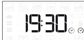
Please note: Programming a delayed cooking start time will disable the oven preheating phase. The oven will reach the temperature you require gradually, meaning that cooking times will be slightly longer than those listed in the cooking table.
