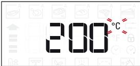
When the °C/°F icon flashes on the display, turn the knob to change the value, then press to confirm and continue with altering the settings for all values that can be regulated.
