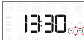
If necessary, turn the *knob* to set the time you want cooking to end, then press to confirm and activate the function.
