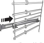
Remove the shelf guides from the oven and remove the protective plastic from the sliding runners.
