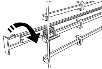
To secure the guide, press the lower portion of the clip firmly against the shelf guide. Make sure that the runners can move freely. Repeat these steps on the other shelf guide on the same level.
