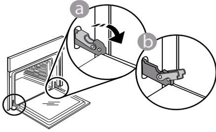
**2.** Close the door as much as you can. Take a firm hold of the door with both hands – do not hold it by the handle. Simply remove the door by continuing to close it while pulling it upwards at the same time until it is released from its seating. Put the door to one side, resting it on a soft surface.
