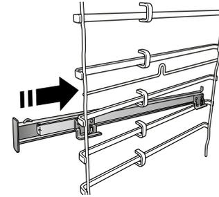
Remove the shelf guides from the oven and remove the protective plastic from the sliding runners. Fasten the upper clip of the runner to the shelf guide and slide it along as far as it will go. Lower the other clip into position.
