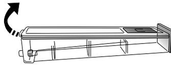
2. Once the cleaning is done, you can close the drawer by inserting the two front flaps inside the front openings and pushing down the back side.
