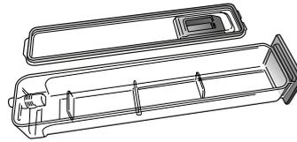
1. Push towards the top the back flap to remove the water drawer top cover.
