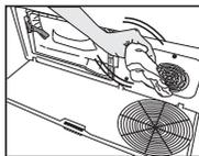
If you see fibre accumulation on the fan cover and the toe board, remove with a cloth.
