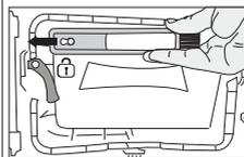
Pull the brush to the left to remove it. You can use the cleaning brush to clean filter, condensing metal surface and accumulated fibre on the door.
