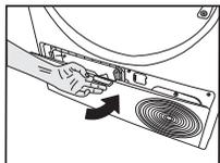
After the cleaning process is completed, place the air deflector cover to its place, move the latches to close it and close the toe board.
