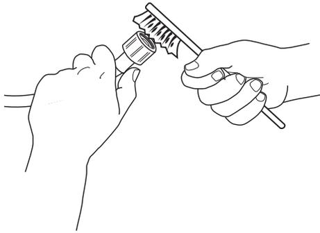
**3.** Now unscrew the inlet hose on the back of the washing machine by hand. Pull out the mesh filter from the valve on the back of the washing machine with pliers and carefully clean it.
