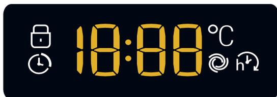
The duration of the available wash cycles and the remaining time of a running cycle appear (the display will show the maximum duration of the cycle chosen, which may decrease after several minutes, since the effective duration of the programme varies depending on the wash load and the settings chosen); if the DELAY START option has been set, the countdown to the start of the selected wash cycle will appear.
