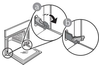
1. To remove the door, open it fully and lower the catches until they are in the unlock position.
