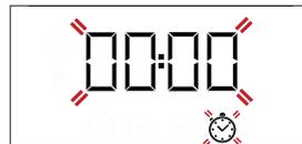
Use + or — to set the time you require and press
