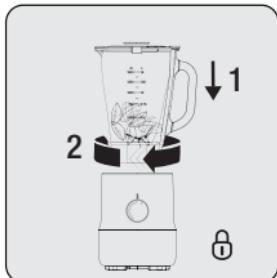
Place the glass container (3) to motor unit (6) upright, turn it to the "0" symbol to lock it in its place.
