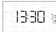
If necessary, turn the knob to set the time you want cooking to end, then press
