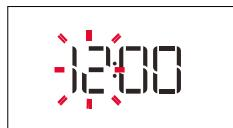
The two digits for the hour will start flashing: Turn the knob to set the hour and press
