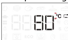
Press or to confirm and start the cooking cycle. During cooking cycle, the display shows meat probe target temperature. When the meat reaches the target temperature set, the cooking cycle stops and the display shows "End". To restart the cooking cycle from "End", by turning the knob it is possible to adjust meat probe target temperature as indicated above. Press or to confirm and restart the cooking cycle.
