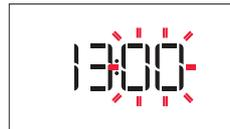
The two digits for the minutes will start flashing. Turn the rotary knob to set the minutes and press
