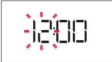
The two digits for the hour will start flashing: Turn the rotary knob to set the hour and then press
