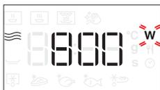
When the icon flashes on the display, turn the rotary knob to adjust the power setting and then press to confirm and continue to alter the settings that follow (if possible).
