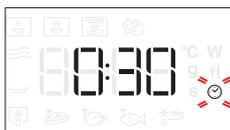
When the icon flashes on the display, use the rotary knob to set the cooking time you require and then press to confirm or press to confirm and start the function.
