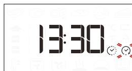
If necessary, turn the knob to set the time you want cooking to end, then press to confirm and start the function.
