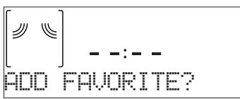
If you would like to save a function as a favorite and store the current settings for future use, press  $\checkmark$  otherwise, to ignore the request press  $\ll$ . Once  $\checkmark$  has been pressed, press + or - to select the number position, then press  $\checkmark$  to confirm.
