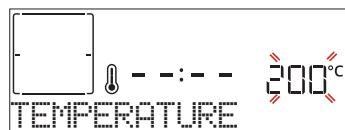
When the value flashes on the display, press + or - to change it, then press to confirm and continue with the settings that follow (if possible).
