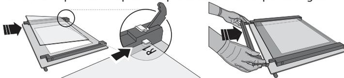
4. Refit the upper edge: A click will indicate correct positioning. Make sure the seal is secure before refitting the door.
