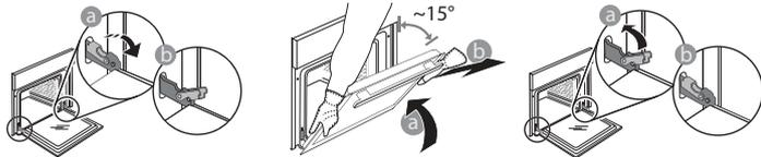
1. To remove the door, open it fully and lower the catches until they are in the unlock position.
