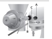
3. Tighten the attachment knob (A) until the unit is completely secured to the mixer.
